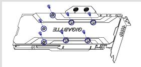
Use the included **7x** M2.5x5 screws and washers (shown in blue) to tighten the block to the GPU core.
