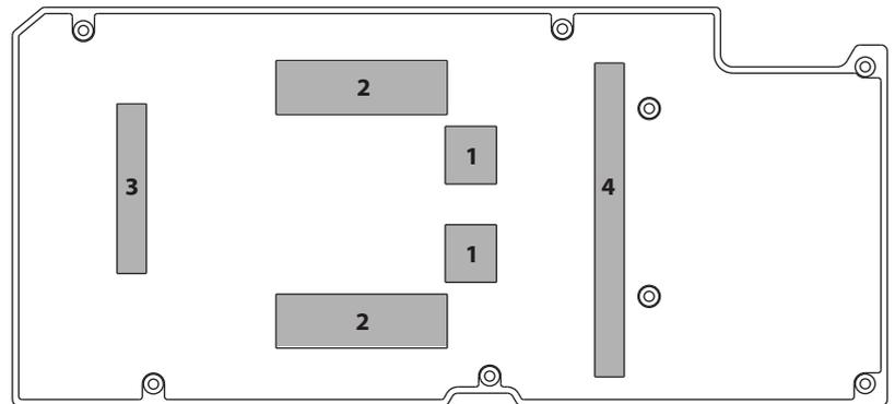
**⚠** Make sure to remove the protective film on both sides of the thermal pads.
